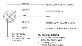
Note: There are internal 10K pull-up resistors from pins 2 and 4 to supply voltage.
