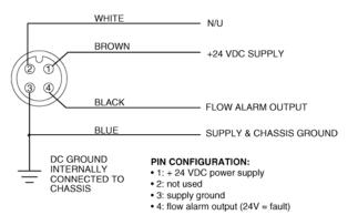
Note 1: Alarm output is driven by an internal solid-state relay (SSR), with a maximum internal "on" resistance of 15 ohms.
