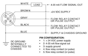
Note: For pulse output, the flow relay contact is closed for 3 msec (pulsewidth)
