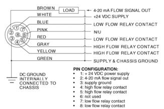
Note: Alarm relays are solid-state (SSR), and have no positive or negative polarity. Maximum internal "on" resistance is 15 ohms
